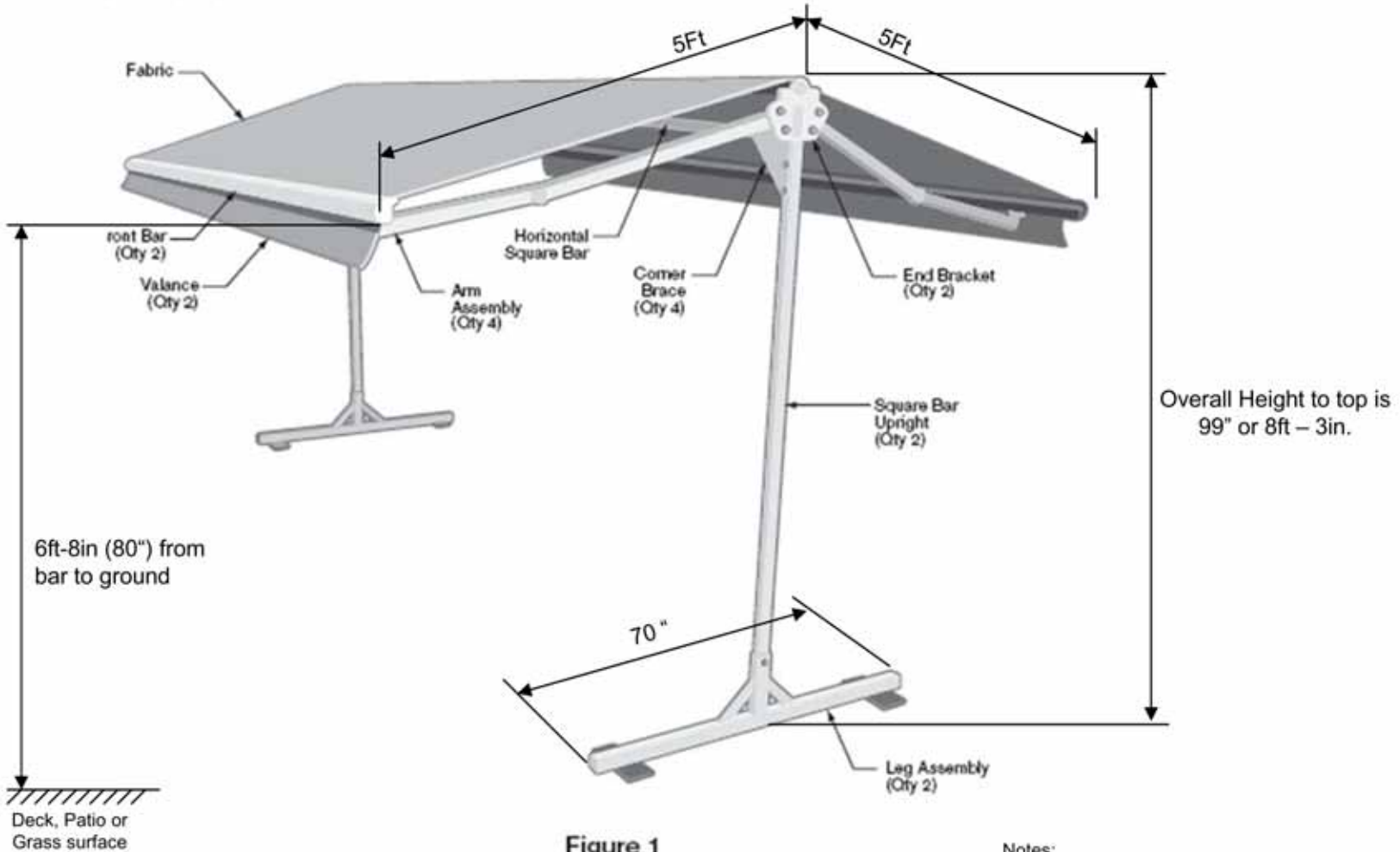
Figure 1 Awning Assembly
